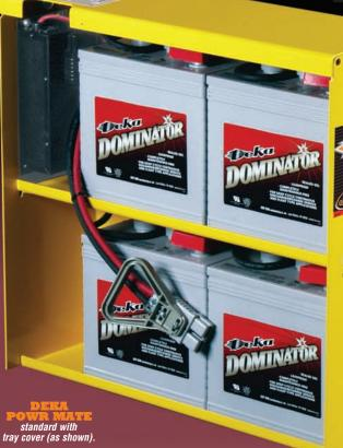
**DEKA POWR MATE BATTERIES** combine all the benefits of a maintenance-free gel battery with an on-board, capacity-matched charger. No need to return the pallet jack to a remote, centralized charging area; simply connect the **DEKA POWR MATE** charger into any 15-amp 120-volt AC outlet.
